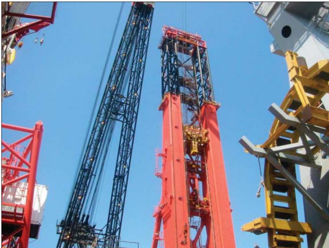
Heerema Marine Contractors used DCV Balder's starboard crane (right) during cross haul and retrieval of Independence Hub's 20-in. steel catenary export riser. The starboard crane includes two traction systems, each with 19 km of steel wire, allowing Balder to manipulate heavy structures at great water depths. Heerema used Balder's 310-tonne capacity mooring line deployment winch (MLDW) for spooling the SCR's cross-haul wire. The yellow piping and structural components in the background are on the topsides of the Independence Hub platform (Fig. 2). Photo by Christopher E. Smith.
