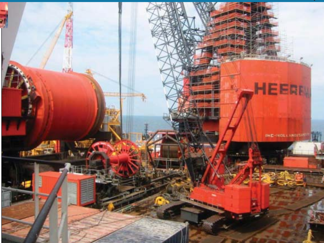
Heerema Marine Contractors used DCV Balder's starboard crane (right) during cross haul and retrieval of Independence Hub's 20-in. steel catenary export riser. The starboard crane includes two traction systems, each with 19 km of steel wire, allowing Balder to manipulate heavy structures at great water depths. Heerema used Balder's 310-tonne capacity mooring line deployment winch (MLDW) for spooling the SCR's cross-haul wire. The yellow piping and structural components in the background are on the topsides of the Independence Hub platform (Fig. 2). Photo by Christopher E. Smith.
